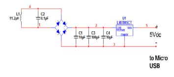
Figure 8. Secondary Circuit
