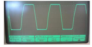
Figure 10. Schmitt Trigger Output
