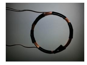
Figure 4. Taped Coil
