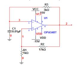
Figure 3. Square-Wave Oscillator
