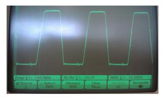
Figure 9. Square-Wave Generator Output
