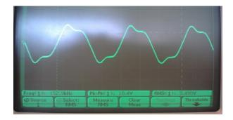
Figure 11. Signal at Secondary Coil
