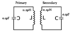
**Figure 5. Parallel Resonant Coils**
